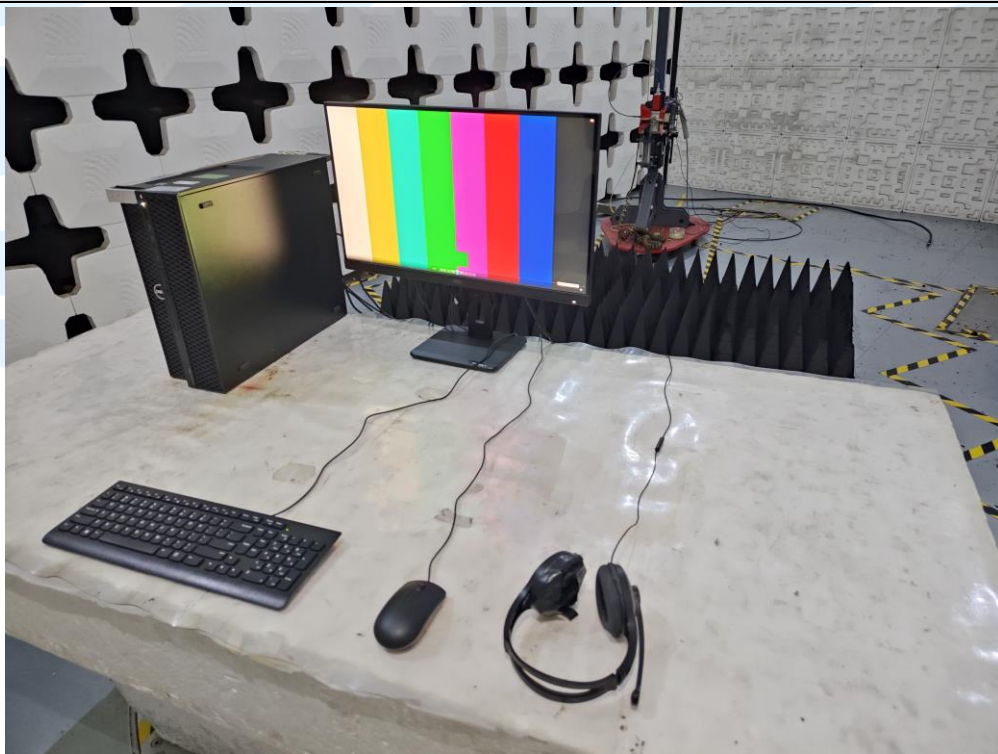
Radiated emission Test Setup (Above 1GHz)
