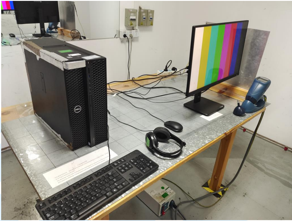
Electrostatic Discharge Test Setup
