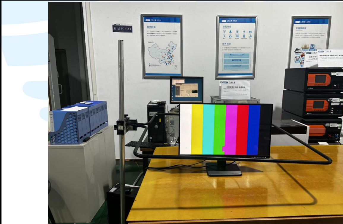
Power frequency magnetic field Test Setup
